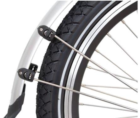
Make sure to check your tire pressure before every ride. Poorly inflated tires are much more likely to suffer a puncture caused by the inner-tube being pinched by the rim.
